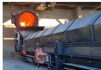
Figure 2, loading of molten slag in Re+Gen®
