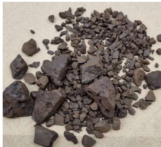
Figure 7, Re+G(arnet)x® samples obtained by cooling black slag via Re+Gen®
