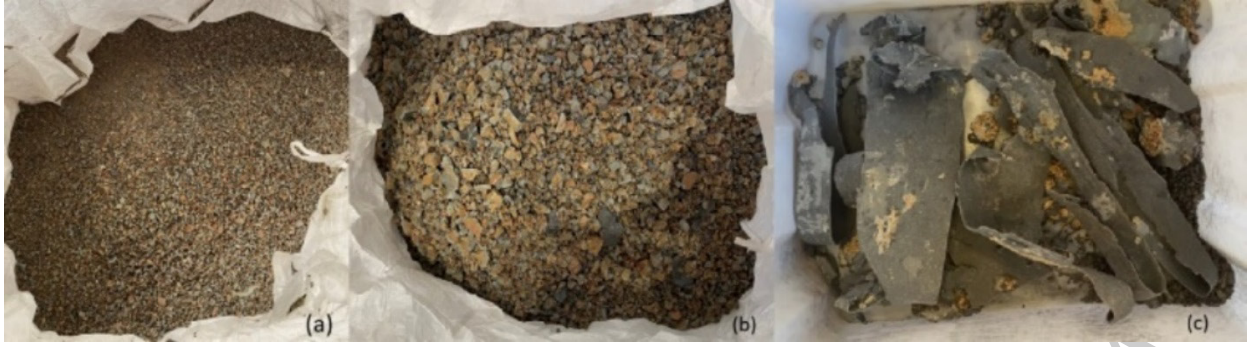
Figure 3, fine fraction of white slag (a), Coarse fraction of white slag (b), recovered metal scrap (c)
