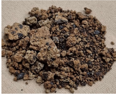
Figure 6, Re+Lime® samples obtained by cooling white slag via Re+Gen®
